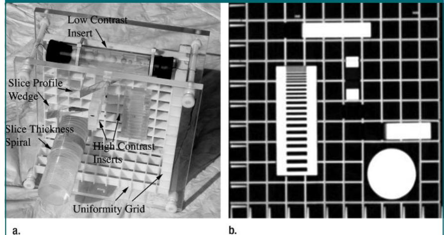
**Figure 1:** (a) High-contrast phantom used to evaluate quality of z-axis reformations by using MTFs. High-contrast inserts are placed at  $90^\circ$  to each other. (b) Representative transverse CT scan of high-contrast phantom acquired at 140 kVp.
