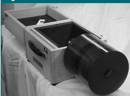
**Figure 2:** Catphan phantom. This phantom contains separate compartments that are used for evaluation of CNR.
